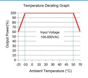
Note 1: The output power should be derated based on the input voltage derating graph at 85~100VAC/850~900VAC. Note 2: This product should operate at natural air condition, please contact us if it need be used at a closed space.
